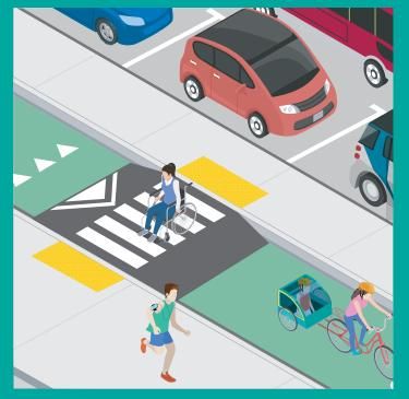
**Figure 24**. Parking-protected cycle track with a raised, wide median that serves as a buffer. Features a raised, high-visibility crossing from the buffer to the sidewalk.
