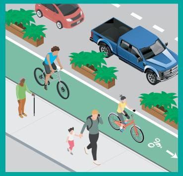
**Figure 27.** Cycle track protected by temporary planters. (*Note: This specific design may not provide sufficient access to the curb.*)
