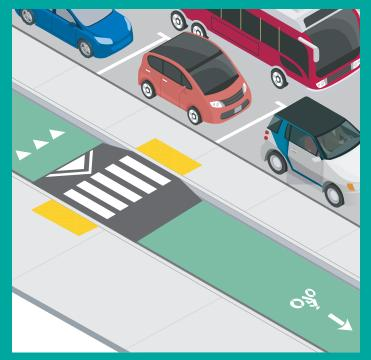
**Figure 23.** Parking-protected cycle track with a wide, unobstructed concrete median.
