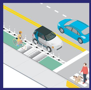
Figure 13. Speed bumps with drainage strips.
