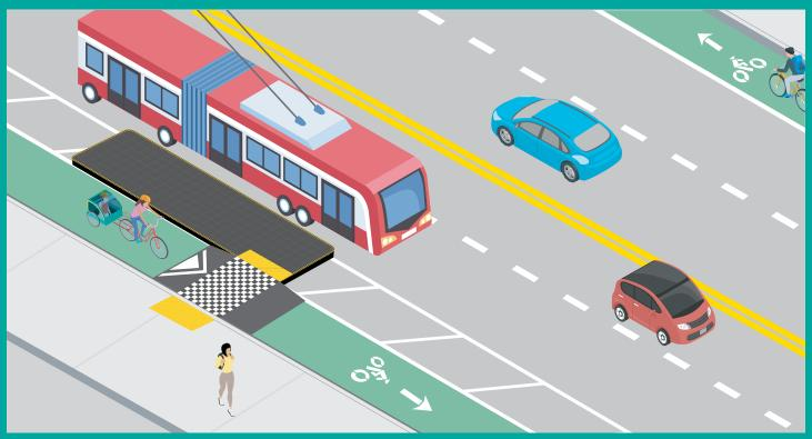
Figure 29. Pre-fabricated transit island that includes a raised cycle track crossing along the sidewalk curb.
