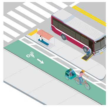
Figure 2. Cycle track protected by a transit island.
