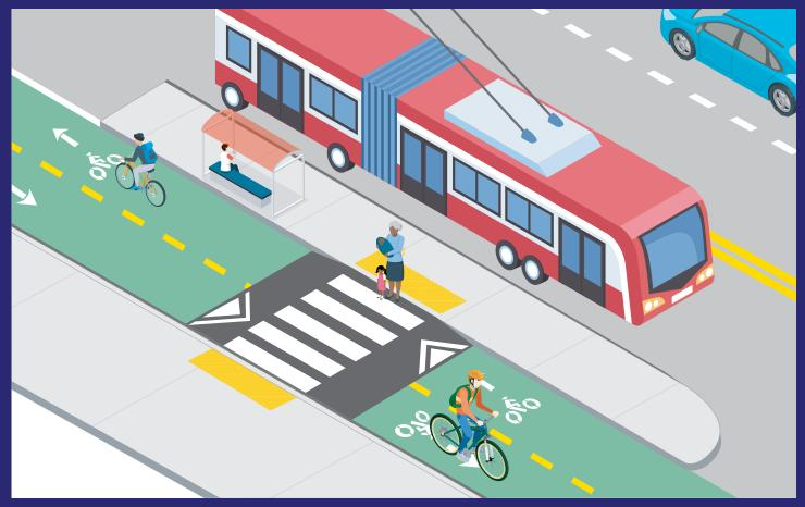
Figure 11. Two-way protected cycle track with a wide raised crossing to a transit island.
