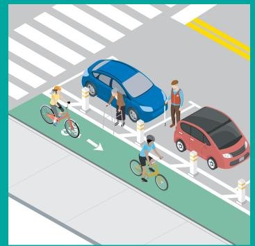
**Figure 6.** Parking-protected cycle track with no ability for people exiting cars to accessibly and intuitively access the curb. Plastic bollards obstruct the "path of travel," forcing those who must access the sidewalk via a ramp to travel in the bike lane.
