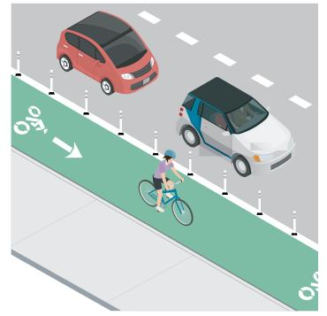
Figure 1. Cycle track protected by soft-hit posts.
