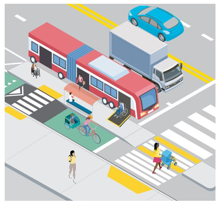
**Figure 26.** Transit island with accessible crossings at both ends of the island. One crossing is raised, which is both accessible and acts as a speed management device for oncoming bicyclists. The second crossing is a ramp that feeds directly to a wide, high-visibility crosswalk and curb ramp.
