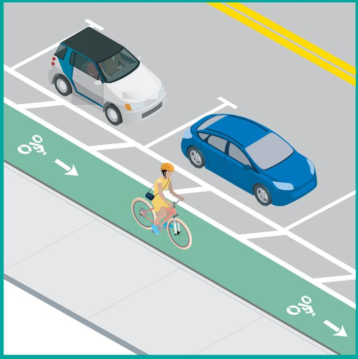
Figure 3. Cycle track protected by parking.
